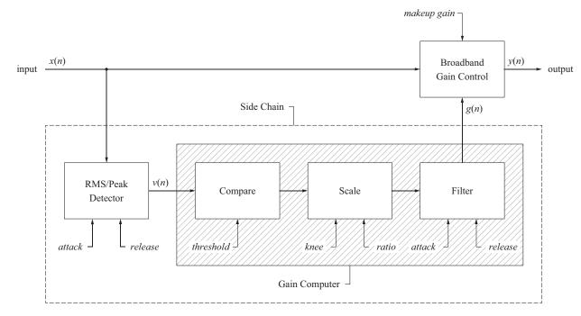
Fig. 1. Basic feed-forward broadband compressor model.
